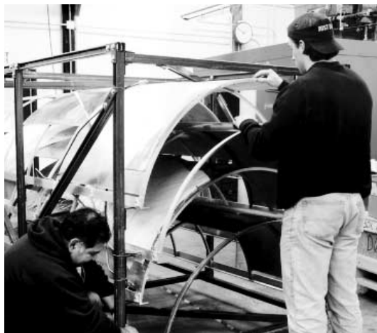
DZero technicians Rolando Flores (left) and Dan Christenson adjust detector parts that will fit between the solenoid and calorimeter.
