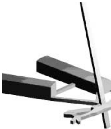
MINOS far detector layout, showing the vertical mine shaft and the detector caverns.
