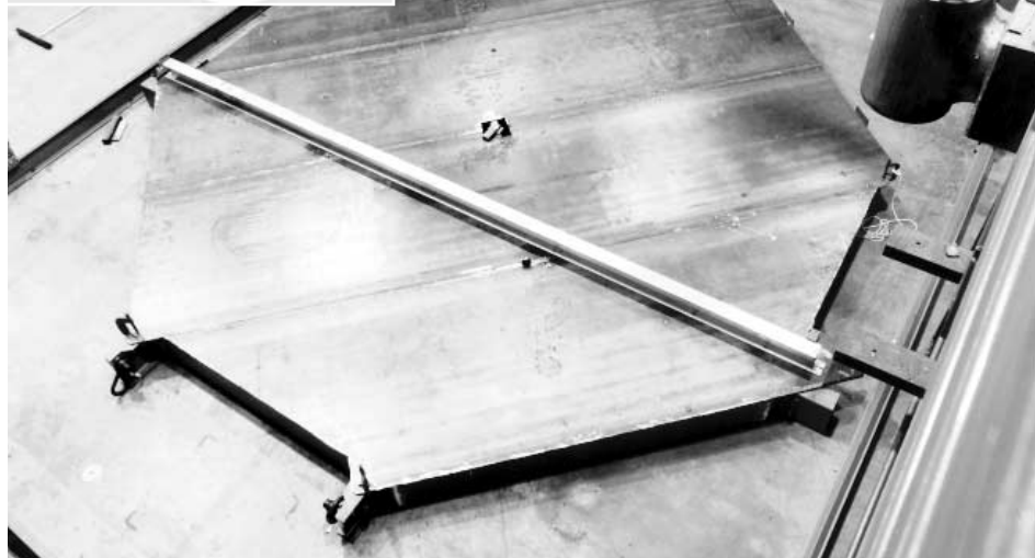
Octagonal steel plates, like slices in a loaf of bread, will alternate with scintillator in the MINOS far detector (inset).
