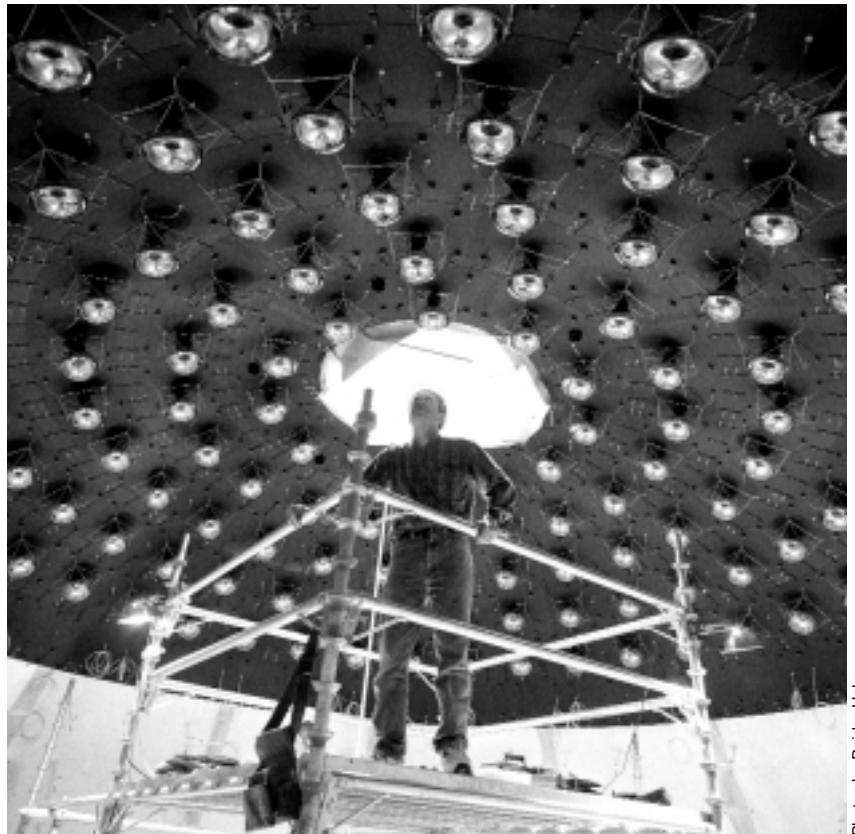
A spherical layer with 1,500 photosensors, mounted on both sides, is placed inside the underground tank of the MiniBooNE experiment.
