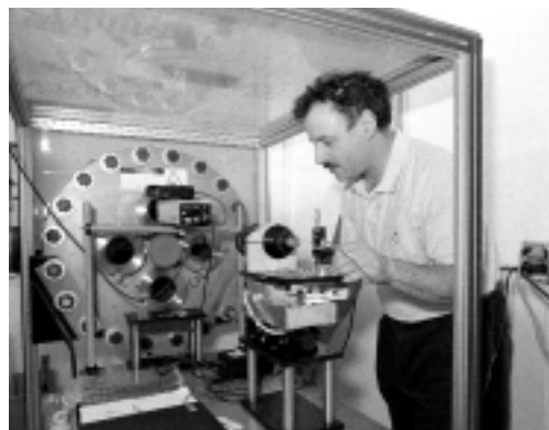
Fermilab engineer Ralph Pasquinelli in the underground enclosures for the laser light link that helps cool antiprotons.
