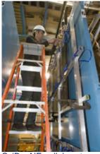
SciBooNE collaborator Yasuhiro Nakajima, a graduate student from Kyoto University, installs counters made up of reused scintillators, photo tubes and bases onto 2-inch recycled steel plates. Other than the support frame, everything in the photo is recycled.
