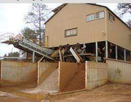
New Riverside Ochre company separates barite of different qualties at its barite processing mill.
