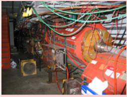
The Injection Region at the Antiproton Source, where newly-made antiprotons are brought to the Debuncher and merged with circulating antiprotons. (Click on image for larger version.)
