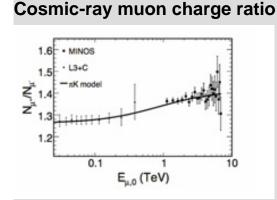
The MINOS collaboration found that the muon charge ratio varies as a function of the muon energy. The black squares represent the MINOS measurements and the triangles represent results by CERN's L3+C experiment.
